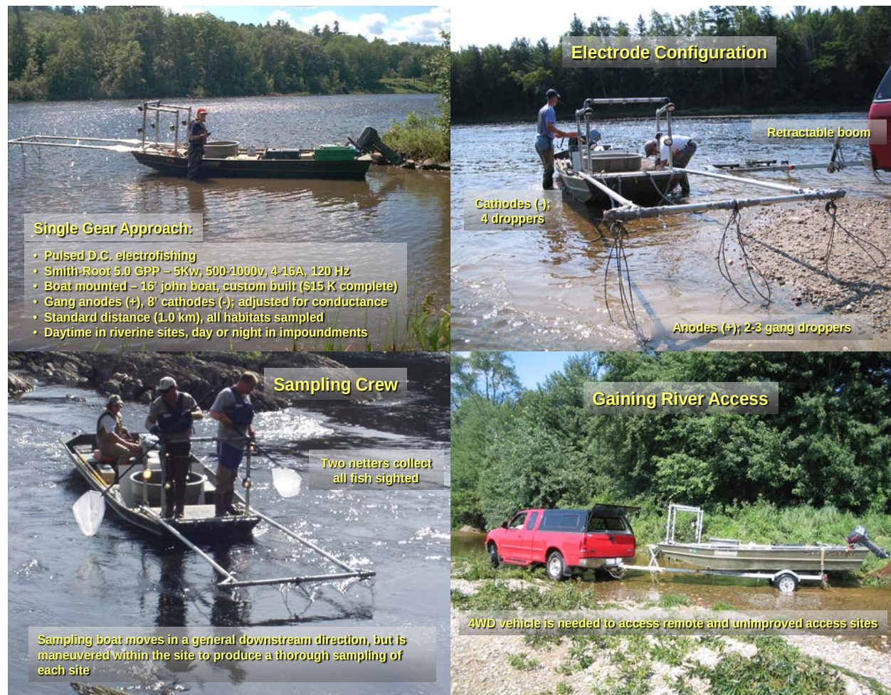
Figure 5. Electrofishing boat and towing vehicle specifications and configuration used in the Maine rivers fish assemblage assessment, 2002-7.
