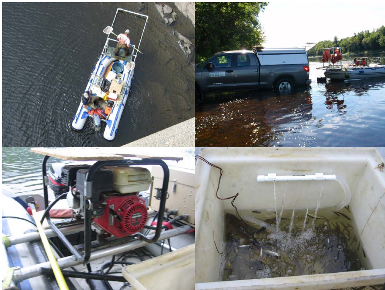
Figure 6. Electrofishing raft details showing boom and frame configuration (upper left), “rough” launching (upper right), GPP generator (lower left), and live well (lower right).
